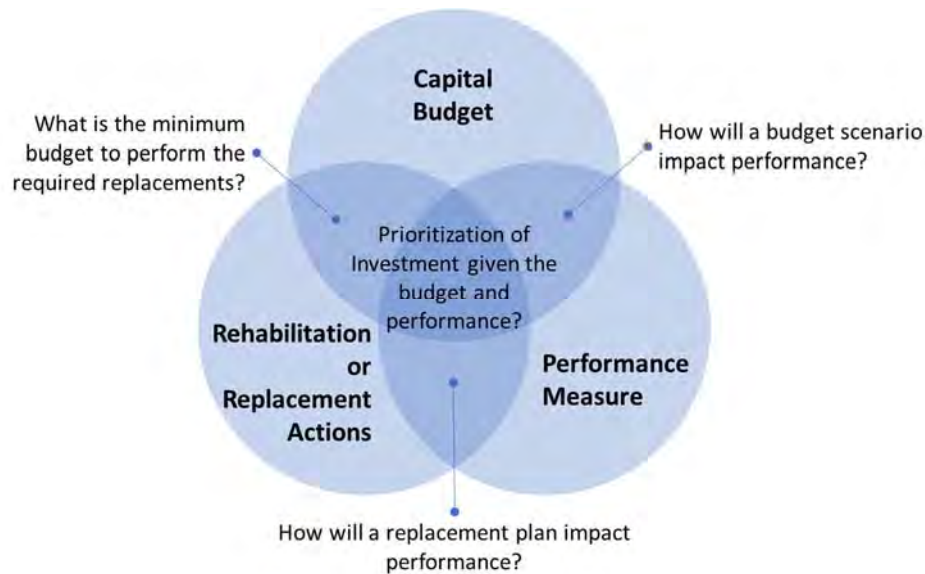
Figure 3. Elements of an SGR Framework to Prioritize Asset Replacement (Adopted from TCRP Report 157 1 )
